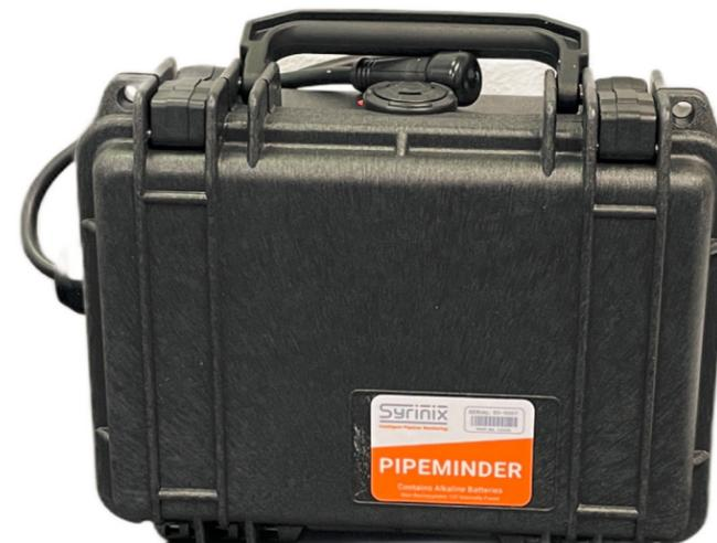
Rechargeable lithium battery typically lasts around 1 year. There is also a 120V w/ UPS power option as well. Typically end users will opt for the re-chargeable lithium battery option and purchase 1 additional battery pack for a swap out program as devices get low with the low battery alert showing up within Radar.
